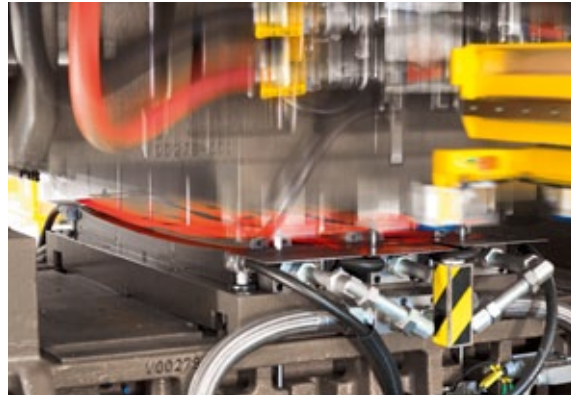
Plasma or gas nitriding can be used on hot stamping tools to further increase hot wear resistance and reduce friction between the tool and sheet materials. Photo courtesy of AP&T Inc.
