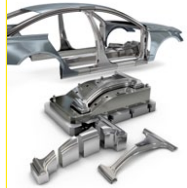
Coatings of PVD type, carried out after nitriding, improve the resistance to abrasive wear and galling.
