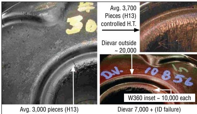
**Figure 7.** The original die obtained an average of 3,000 pieces. When heat treatment was enhanced, the average went up to 3,700 pieces. The use of Dievar for the entire die resulted in over 7,000 pieces before wear and cracking occurred. By using Dievar for the outer die and inserted with W360 Isobloc, the average went up to over 10,000 pieces.
