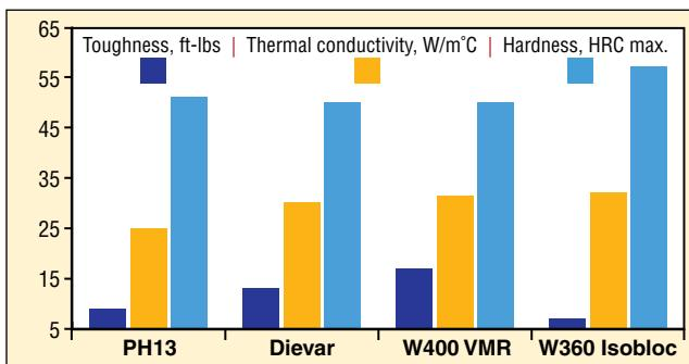
Figure 2. Thermal conductivity, toughness and hardness of several new tooling grades. Thermal conductivity is taken at room temperature.
