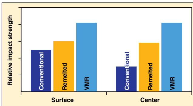
Figure 1. Comparison of ductility of tool steel as a function of steel production method. VMR indicates vacuum melted remelted steel. Note the uniformity between surface and center for the remelted and VMR processing methods.
