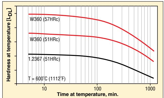
Figure 5. W360 Isobloc hardness as a function of time at 600°C (1112°F). Even at a lower hardness of 51 HRC, the material will not soften below the initial hardness until 800 minutes, versus that of 1.2367, which begins to soften below 51 HRC at 40 minutes.
