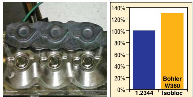
Figure 6. Example of forging die showing a substantial improvement in die life.
