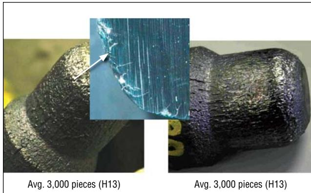
**Figure 8.** Improvement in punch life using a conventional 1.2367 alloy.
