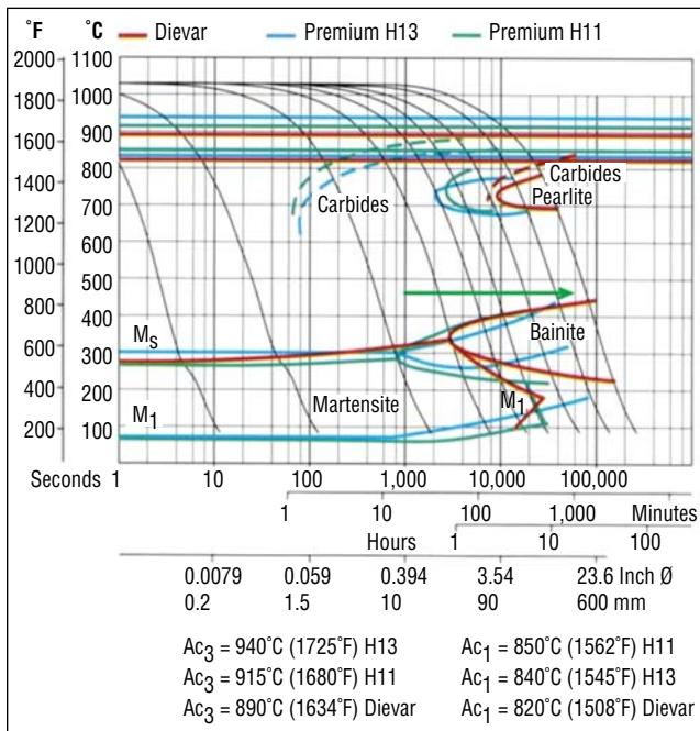
Figure 4. CCT curves for Dievar, Premium H13 and Premium H11. Carbide and bainite noses are pushed out in time for Dievar, for increased cooling time.
